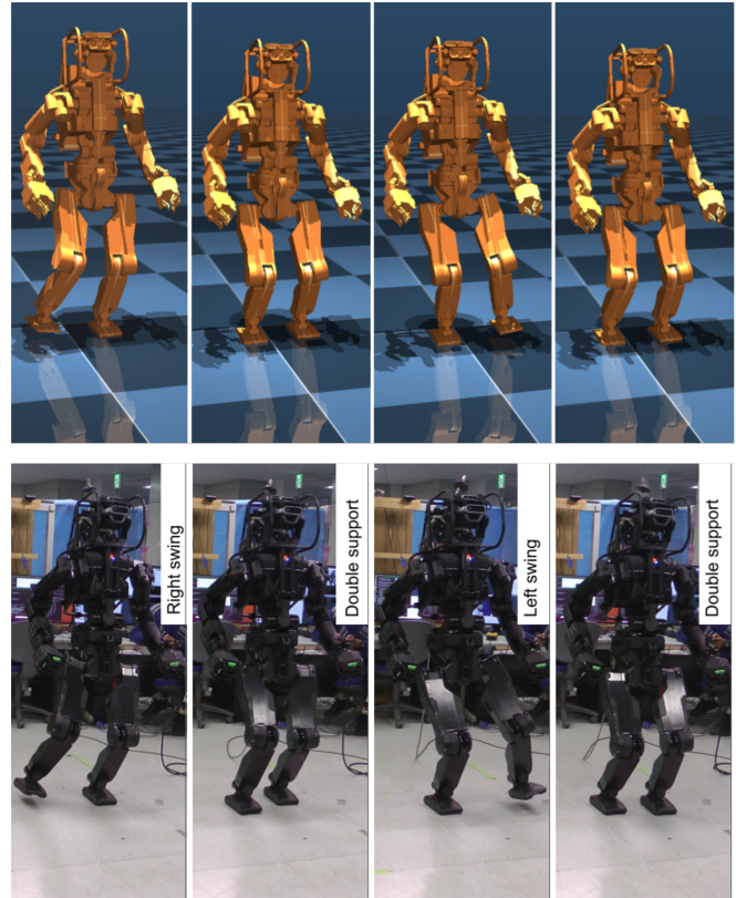
Fig. 1: HRP-5P humanoid robot trained to perform bipedal locomotion via model-free reinforcement learning in MuJoCo (top); RL policy transferred to the real robot (bottom). We make use of the feedback from measured actuator current to account for the poor torque tracking on the real system.
