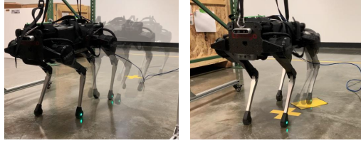
Figure 6: Real robot tests. Left: Timelapse of forward walking. Right: The left rear leg is perturbed.
